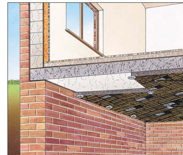
FOAMGLAS® Wallboard/slab T4 WDS fixed by adhesive 2 Mechanical fixings
