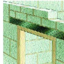
Coursing Bricks can be used as in-fill around doors and windows to avoid cold bridging and protect against pattern staining on internal walls.
