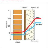
EVT structures comply with the EVT Standard. They combine high levels of insulation with the ability to ensure any natural moisture ingress into the structure always migrates safely and
