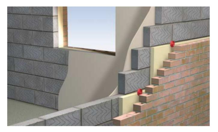
Thermalite Turbo building block offers very high thermal insulation properties and is therefore ideal for external wall applications where low U-values are required.
