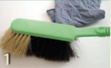
All surfaces must be stable, dry, smooth and free of dust, silicone and grease. Brush down all surfaces and vacuum clean or wipe with a cloth if necessary. On sanding plaster or surfaces with very fine dust it may be necessary to prime the surface with BUDAX AC.
