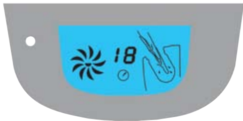
Biodrier Business - CPU controlled with an LCD display, counting down from 18 to 0 seconds.
