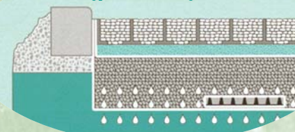
Figure 2 Typical Infiltration System
